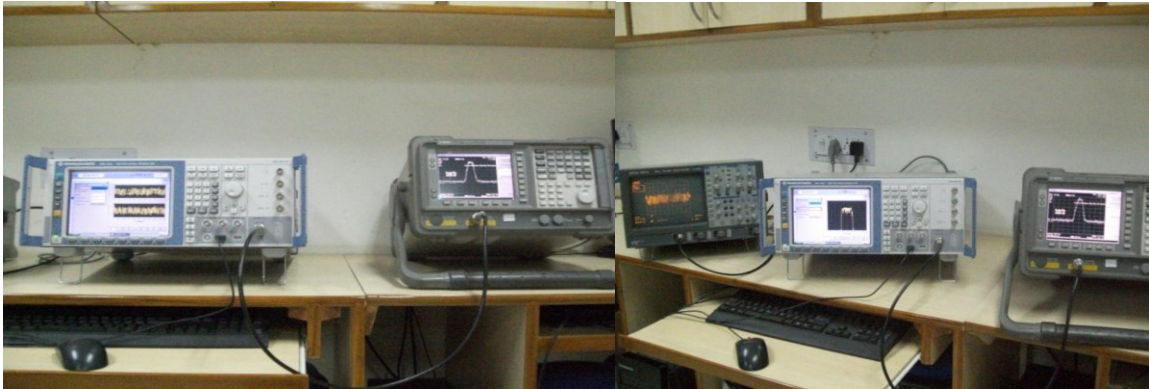
Vector Signal generator and Spectrum Analyser
